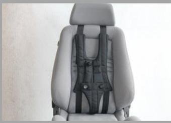
Place the harness pad against the seat backrest, place shoulder straps with triangular assembly plate to the rear of the seat backrest, feed these below the headrest of the seat. Place the lower triangular assembly plate with the lap and crotch straps through the gap at the bottom of the backrest.
