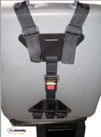
Position the triangular assembly plate high on the back of the backrest, close the buckle and adjust both shoulder belts. This is done by tightening the belt on the triangular assembly plate.
